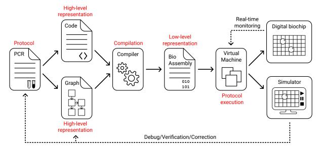
Figure 1: Overview of the main steps of the programming environment starting from the definition of the protocol and terminating with the execution on the biochip. The simulator is used to debug, verify, and correct the protocol.
