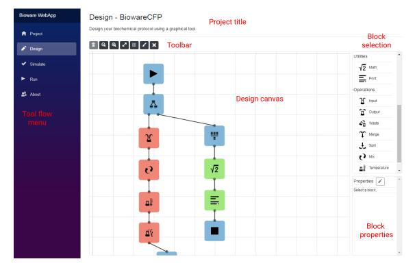
Figure 3: The web-based interface for designing a protocol using an intuitive high-level block-based representation. Blocks correspond to classic programming operations (arithmetics, flow control, printing, etc.) and fluidic operations (dispensing, mixing, incubation, temperature control, sensing, etc.).
