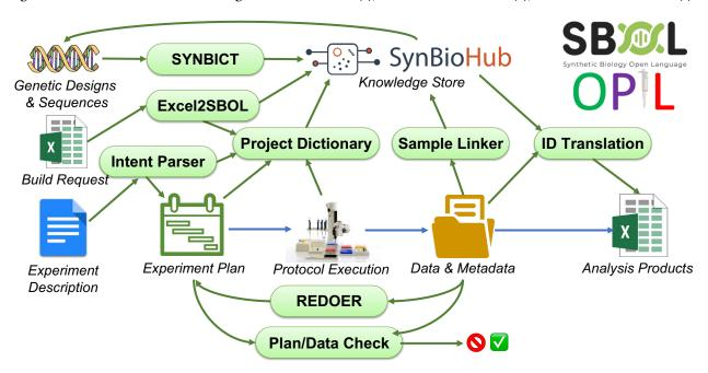
Figure 2: High-level diagram showing how data representation tools were deployed in the DARPA SD2 program with respect to inputs of designs, build requests, and experiments requests, and outputs of data, metadata, and analysis products. This diagram focuses specifically on the key representations (SBOL and OPIL) and representation-centric tooling, and not other aspects of supporting automation used in SD2.
