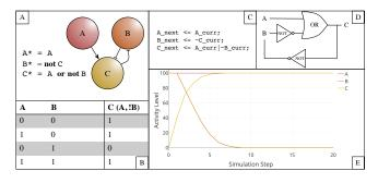
Figure 1: (A) A graphical representation of a simple toy Boolean model with three elements, as well as the Boolean expressions for the next state (\*) for each element. (B) The truth table for the value of Element C. (C) SystemVerilog logic statements. (D) Logic gate representation of the toy model. (E) Simulation results using the DiSH simulator [9], a software-based simulator.
