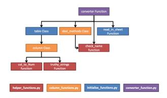
Figure 3: The module architecture of the Excel2SBOL Python Package. Note that the colors of the functions indicate which Python module they can be found in, as indicated in the key on the bottom right.
