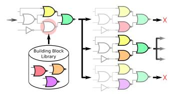
Figure 2: Excerpt of Branch and Bound's search tree for an exemplary circuit. The marked gate is systematically assigned library gates and resulting partial mappings are scored with the bounding function, i.e. simulated with optimistically estimated inputs. Inferior partial solutions are then pruned, while here, one solution is expanded further.
