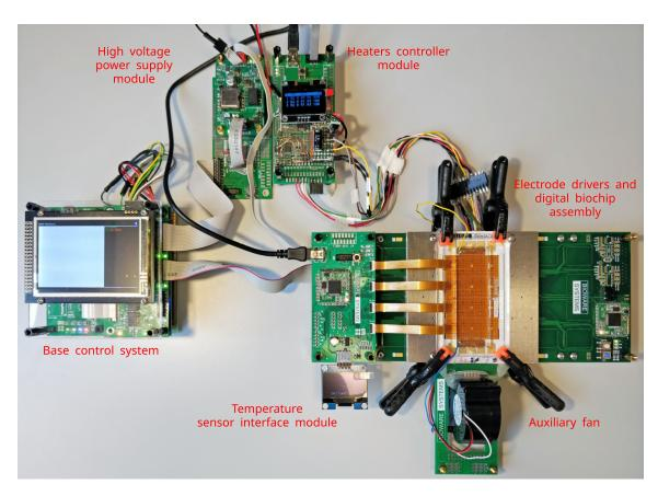
Figure 2: The BiowareCFP configured for temperature calibration of three temperature regions used for the annealing, melting, and elongation steps of the PCR protocol.
