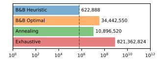
Figure 3: Number of simulations needed for mapping the set of 66 benchmark circuits with the examined algorithms.
