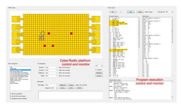
Figure 4: The graphical user interface of the virtual machine executing a testing protocol where droplets are sorted based on their color. The interface allows users to monitor and control the protocol execution and the cyber-fluidic platform.
