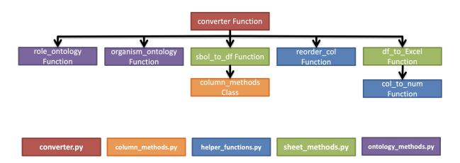
Figure 2: The module architecture of the SBOL2Excel Python Package. Note that the colors of the functions indicate which Python module they can be found in, as indicated in the key on the bottom right.
