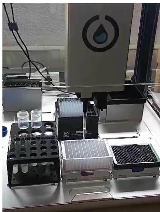
Figure 3: Opentrons OT-2 liquid-handling robot. The OT-2 is already prepared to execute the protocol with all the labware in the right position. The pipettes used are the Multichannel P300 on the right mount and the Single Channel P1000 on the left mount.
