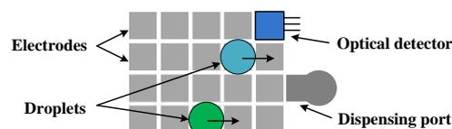
Figure 1: Schematic view of a digital microfluidic biochip.
