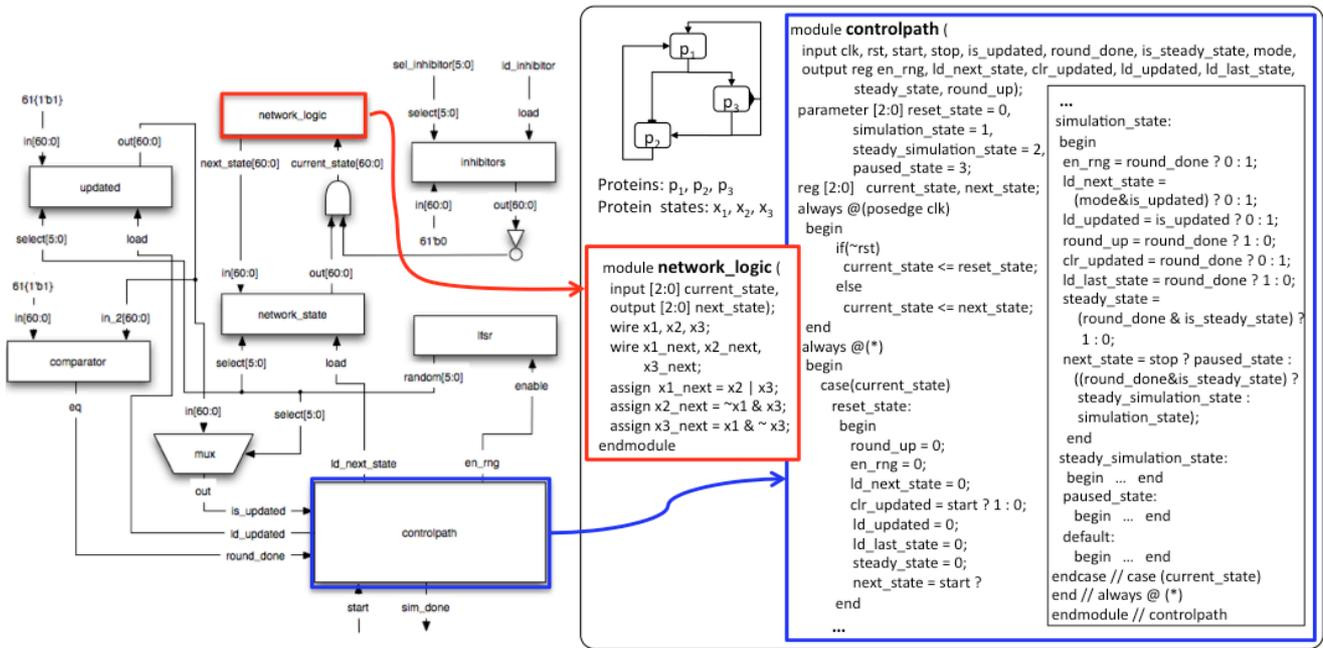
Figure 1. Designed circuit modules (left) and Verilog implementation (right) of two modules: `network_logic` module for the example network and `controlpath` module.
