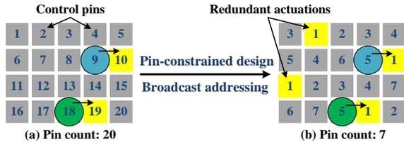
**Figure 2:** Moving two droplets in a specific time step. (a) A direct-addressing result uses two pins (pin 10 and pin 19) to generate two exact actuations. (b) A broadcast-addressing result uses one pin (pin 1) to generate two exact actuations, plus two redundant actuations.
